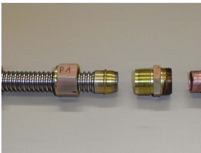
Figure 7: (after test) Sample P1 opened. No visible signs of deterioration that could indicate reduced lifetime or leakage
